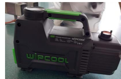
Vacuum pump for the field water filtration
